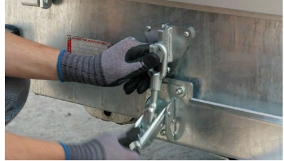
Figure 1: Front beam latches
